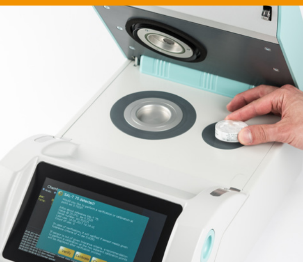
Left: Simple traceable calibration with RFID re-useable salt capsules. By swiping the salt over the chip reader, the calibration is automatically started.
