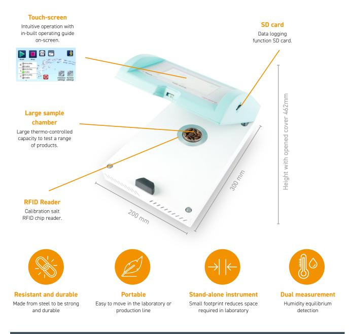
Fully compliant with ISO 18787: 2017 water activity testing standard
