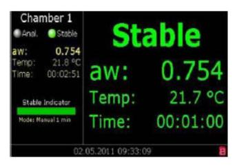
Fast and precise aW-measurement thanks to the worldwide unique "Novalyte" measurement technology CM2 sensor
