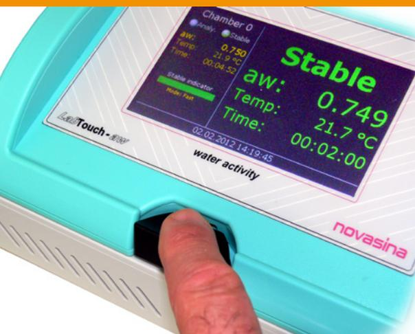
Left: Simple traceable calibration with RFID re-useable salt capsules. By swiping the salt over the chip reader, the calibration is automatically started.
