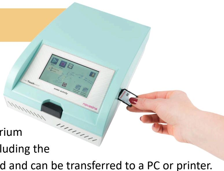
***The LabTouch-aw excels with speed, high measurement accuracy, reproducibility and robustness. Consequently, this system sets new standards for aw-value measurement. Supplied complete with calibration standards and epw sample cups.***
