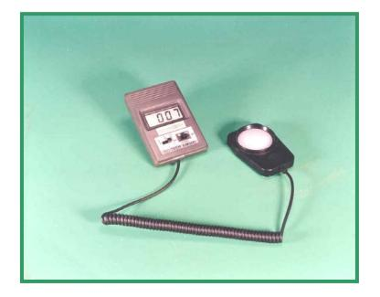
The Novatron Lux Meter is designed to give light level readings up to 50,000 lux. It has a sensor connected to the meter by one metre of coiled lead (when extended). This allows light measurements to be made away from the subject area, thereby minimising errors due to shadow, etc.
