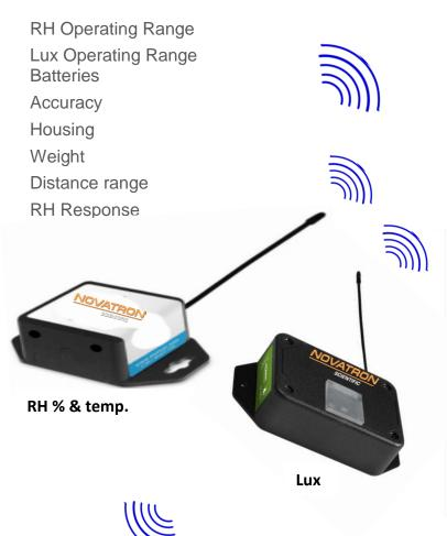
0 – 100% RH & 0-50 C 0-1000 Lux 2 x AA alkaline, lasting around 3 years +/- 3% & 0.5 C @ 10% - 90% RH. +/- 5% Lux
