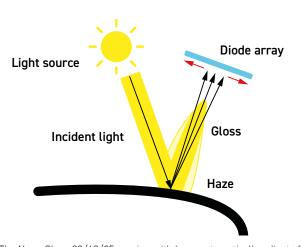
The Novo-Gloss 20/60/85 version with haze automatically adjusts for non-flat surfaces by sensing the reflected peak and virtually adjusting the position.
