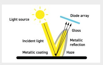
The Novo-Gloss 20/60/85 version with haze captures compensation information from a region adjacent to the haze measurement angle. This means it can be used on metallic coatings which reflect light.
