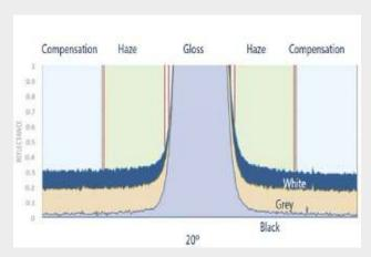
Goniophotometric information profiling the reflection from white, grey and black panels with an identical topcoat.
