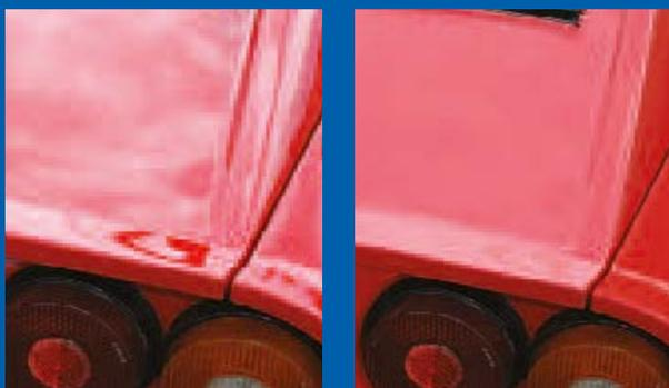
The gloss of a surface can be greatly influenced by a number of factors, for example the smoothness achieved during polishing, the amount and type of coating applied or the quality of the substrate.
