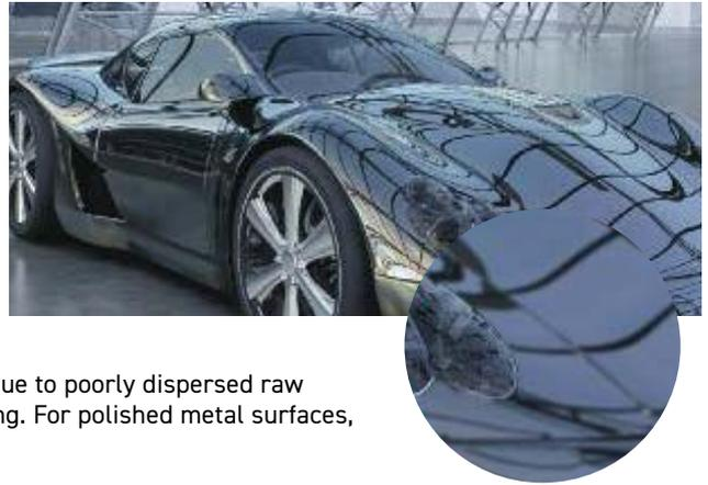
In the coatings industry, this microscopic surface texture is often due to poorly dispersed raw materials, incompatible raw materials or oxidation and weathering. For polished metal surfaces, haze is often associated with polishing marks or chemical residue.
